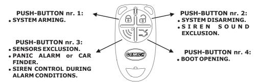
When batteries are almost uncharged, the LED will flash at every pressing of the radio control push button.
